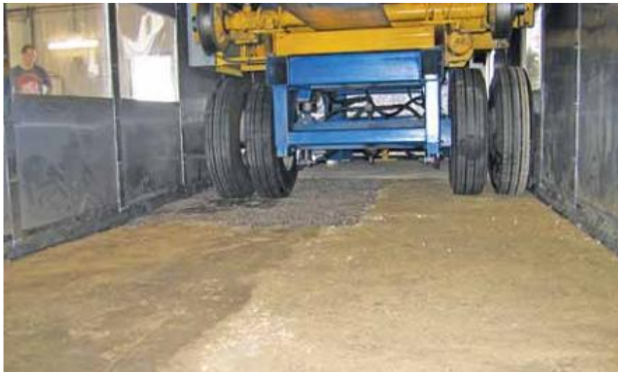
Figure 6. Moving wheel test (from Pokharel [8])
