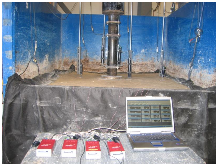
Figure 4. Cyclic plate loading test
