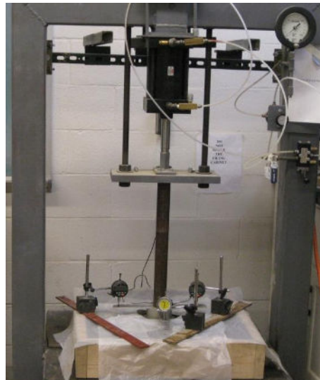
Figure 1. Static plate loading test
