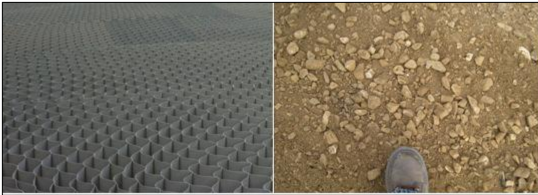
Figure 2: Neoloy and Gravel Infill Material
