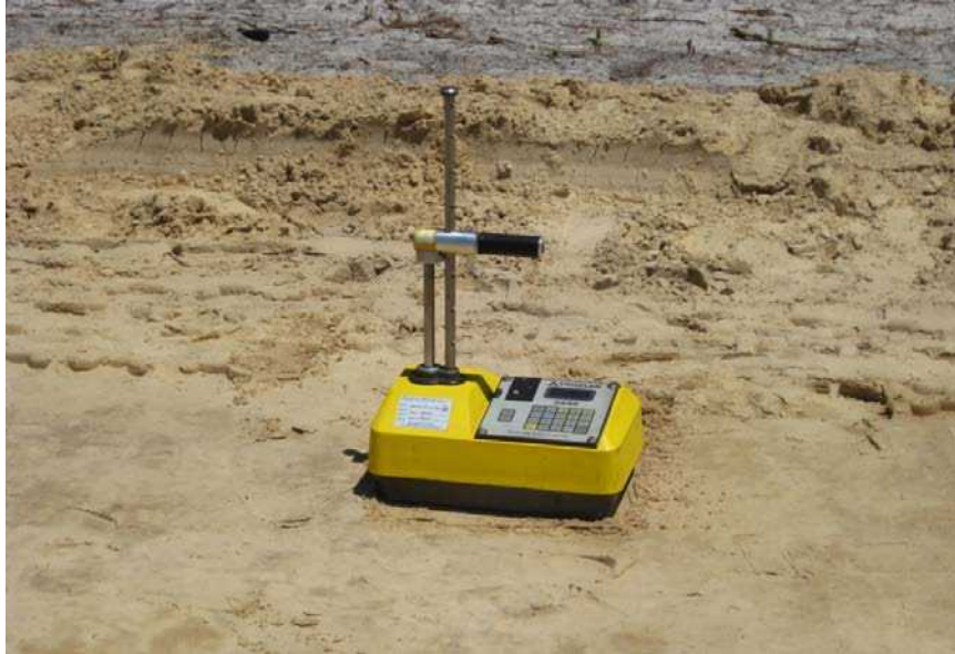
Figure 12. Troxler nuclear gauge used for moisture and density testing
