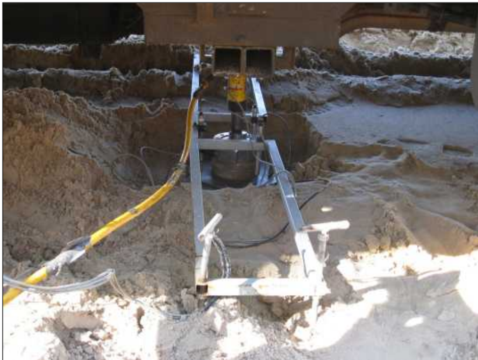
Figure 9. Static plate load testing (PLT) setup using freightliner, reaction beam, and 300 mm diameter steel plate, and 3 deflection sensors
