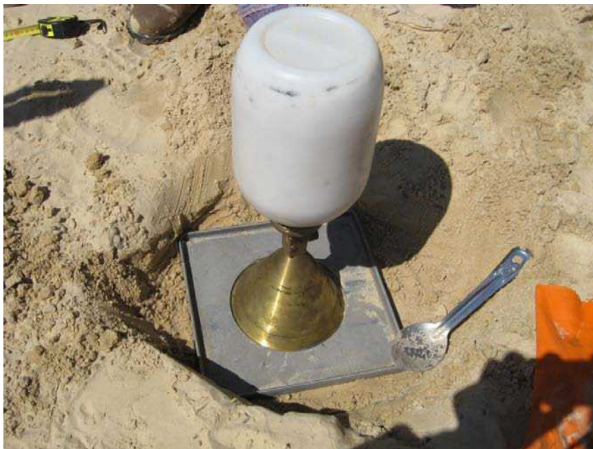
Figure 13. Sand cone testing used for moisture and density determination
