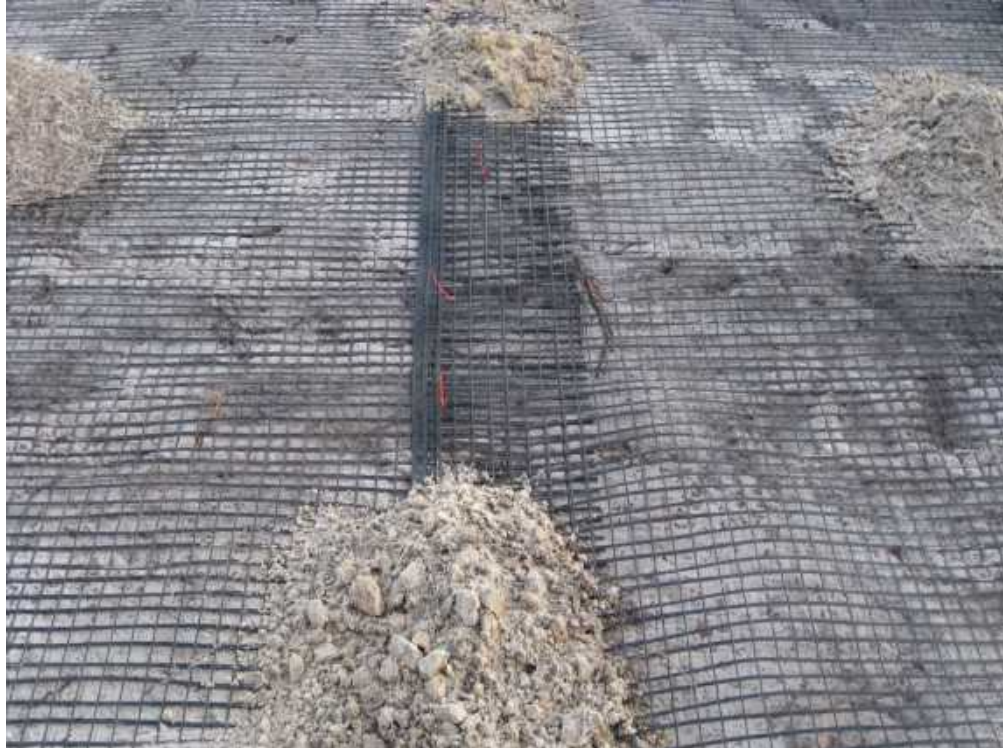
Figure 3. Pictures of BX geogrid used in this study
