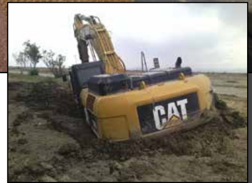
Above: Partially infilled NPA geocell road construction over clay mud swamp. Inset: Heavy construction machinery sinking in airport's soft clay mud (no NPA geocell reinforcement). Photo credits: Innovater
