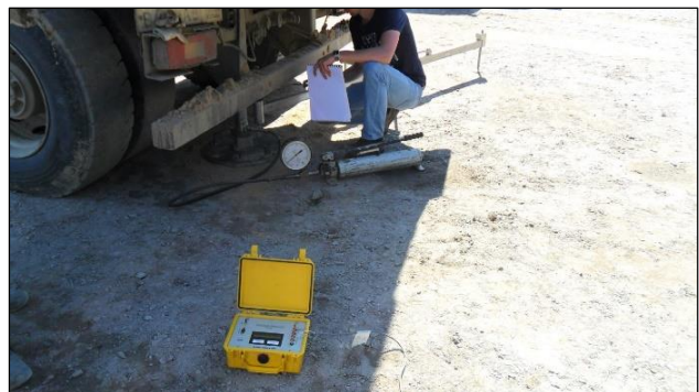
Figure 1. Plate load testing on surface of granular layer
