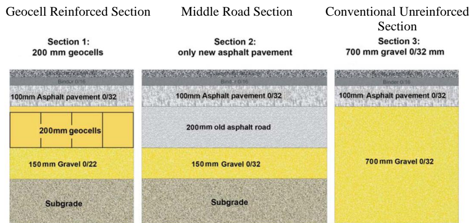
Figure 3: Graphical representation of the different rehabilitated road sections
