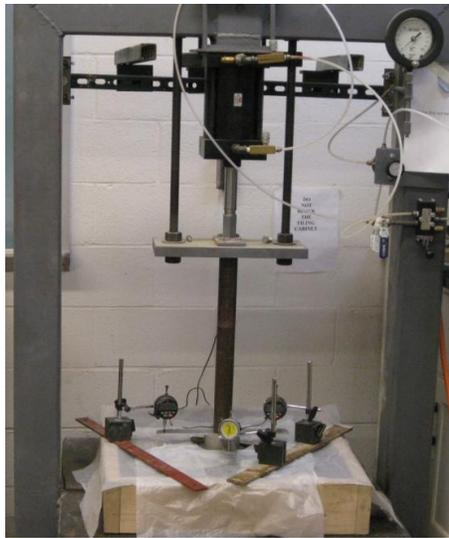
Figure 1. Static plate loading test
