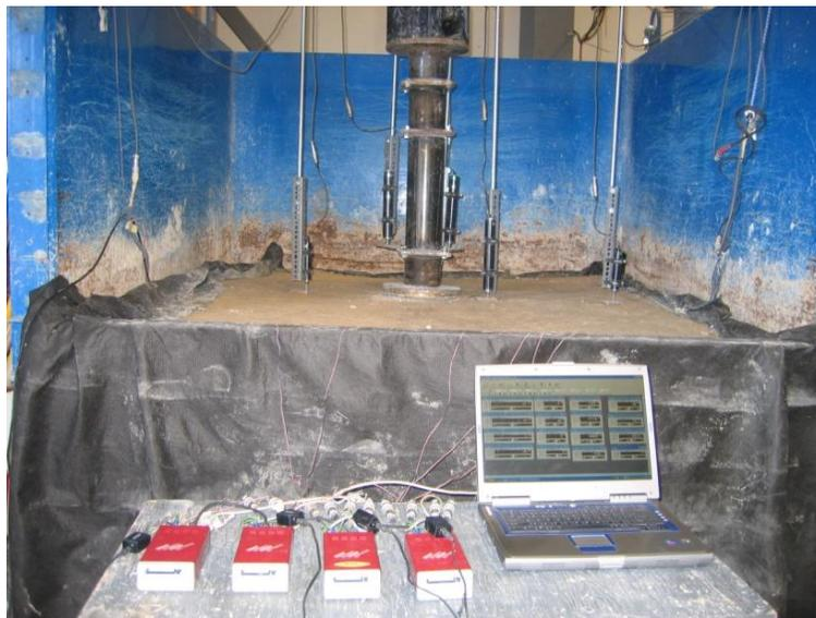
Figure 4. Cyclic plate loading test
