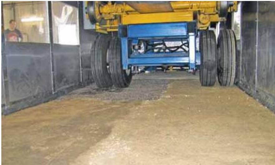
Figure 6. Moving wheel test (from Pokharel [8])
