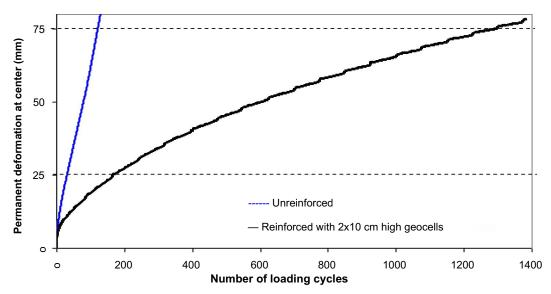
Figure 1. Effect of Geocell reinforcement on pavement permanent deformation (reproduced from Pokharel, 2010).
