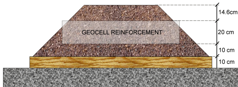
Figure 4. Single-layer reinforced test cross-section.
