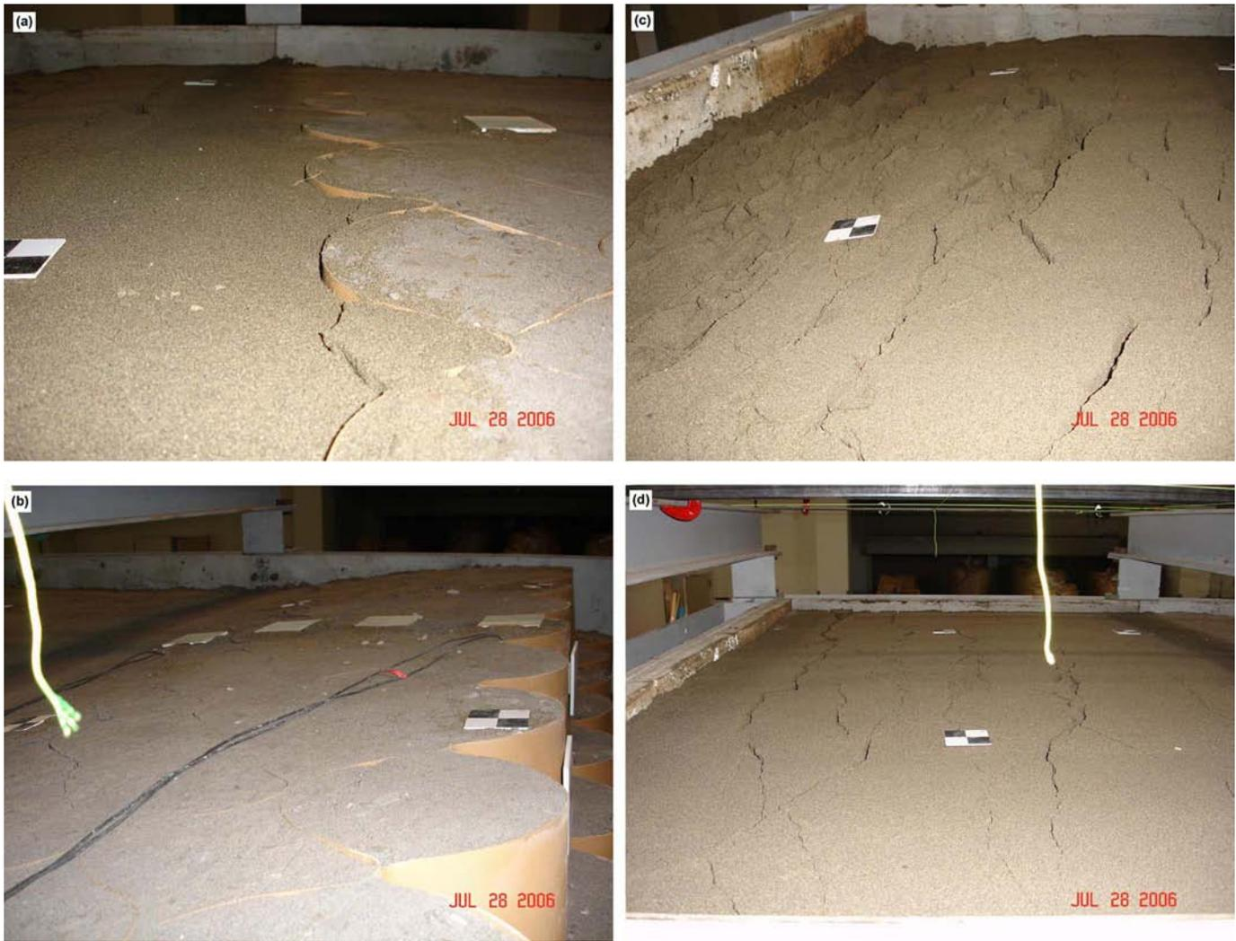
**Fig. 10.** Surface settlements and cracks in Wall 3 after the third shaking: (a) settlement behind the long geocell layer; (b) differential settlement between the geocell facing and backfill; (c) surface cracking in the backfill; and (d) surface cracking in the backfill after the second shaking
