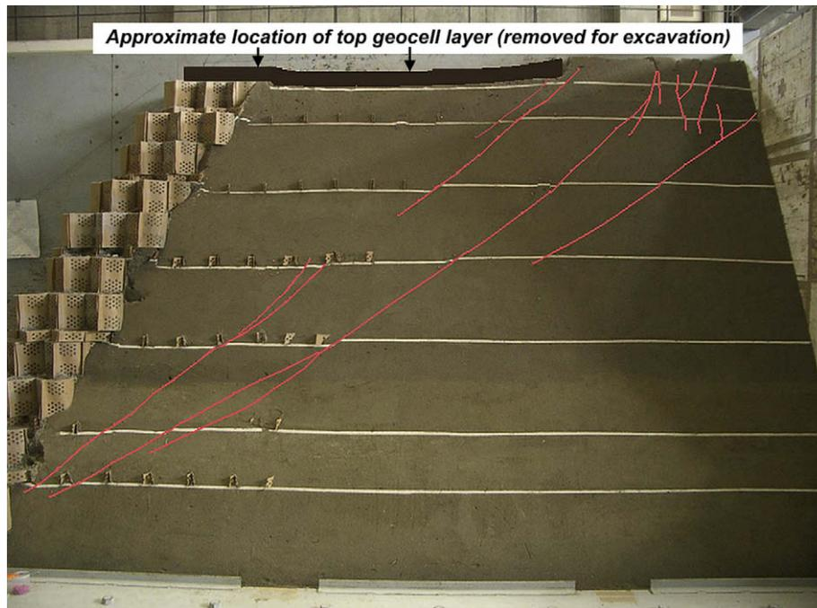
Fig. 9. Excavated section: Test 5 (PGA = 205% of Kobe's).
