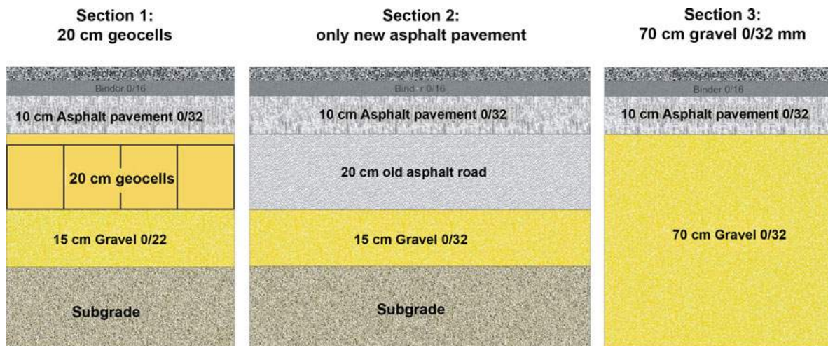
Figure 4: different reconstruction section, road K-23
