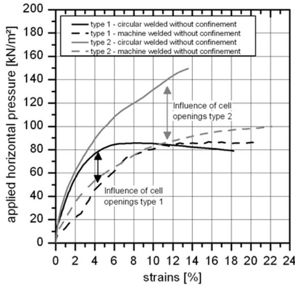
Figure 3: comparison between circular and machine welded geocells
