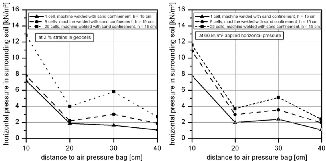
Figure 7: distribution of measured horizontal pressure in soil depending on the number of adjacent cells
