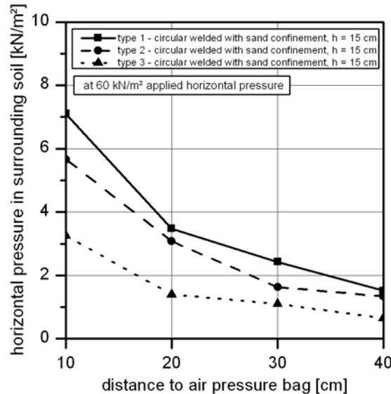
Figure 5: distribution of measured horizontal pressure in the surrounding soil depending on the stiffness of the geocell material
