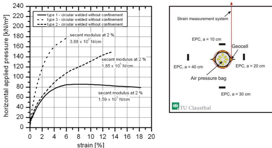
Figure 2: pressure-strain curves for different geocell materials without soil confinement
