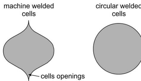
Figure 1: Different forms of tested geocells
