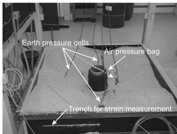
Figure 2: Radial load test (RLT) device
