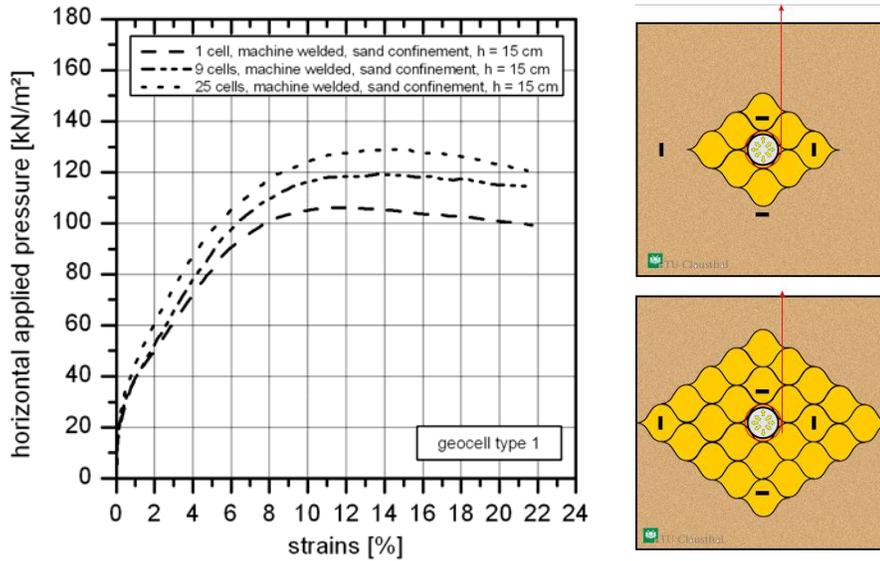
Figure 6: pressure-strain curves depending on the number of adjacent geocells
