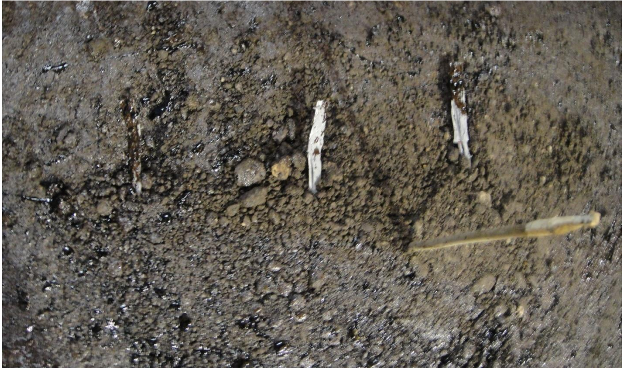
Figure 4.4 Prime coat on the RAP base with the tell-tale and pavement strain gauges
