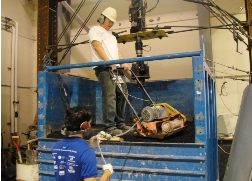
Figure 4.5 Compaction of the HMA surface by the vibratory plate compactor
