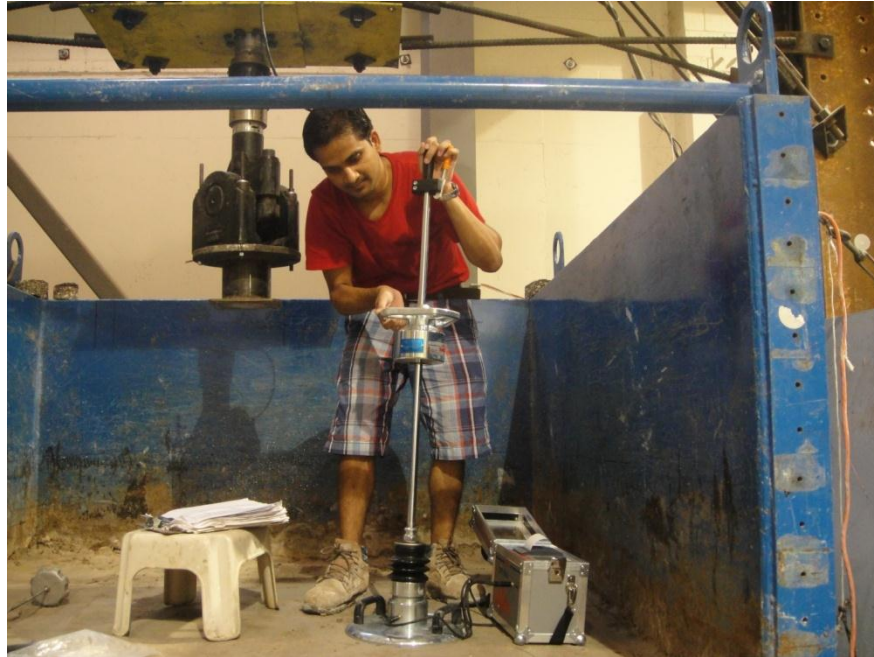
Figure 3.15 Light weight deflectometer test on the prepared test section
