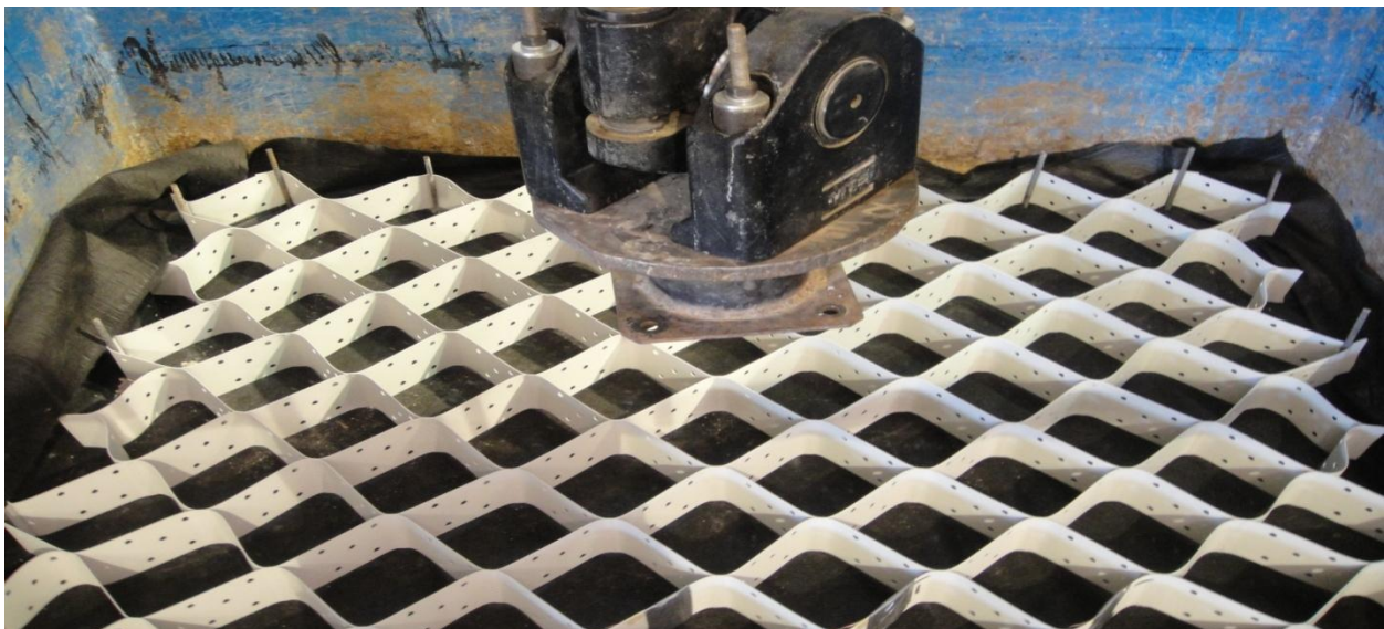
Figure 4.2 Geocell installed on the geotextile over the subgrade
