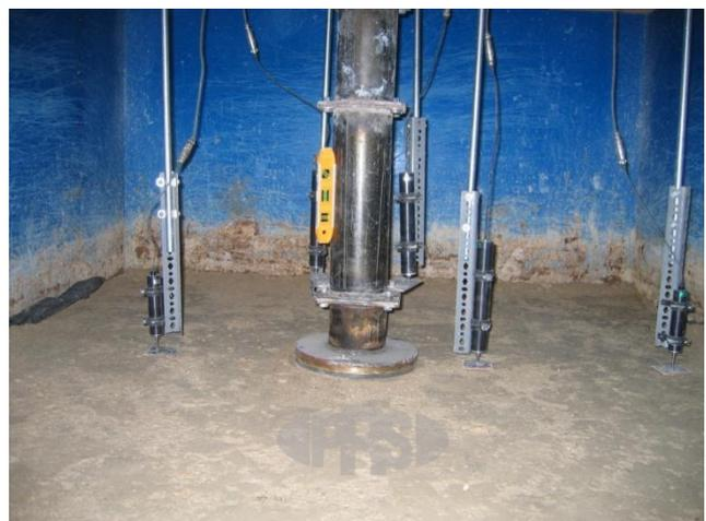
Figure 03. Large-scale plate loading test in the geotechnical test box at the University of Kansas
