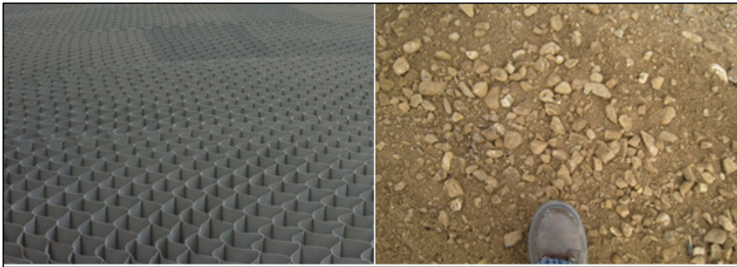
Figure 2: Neoweb and Gravel Infill Material
