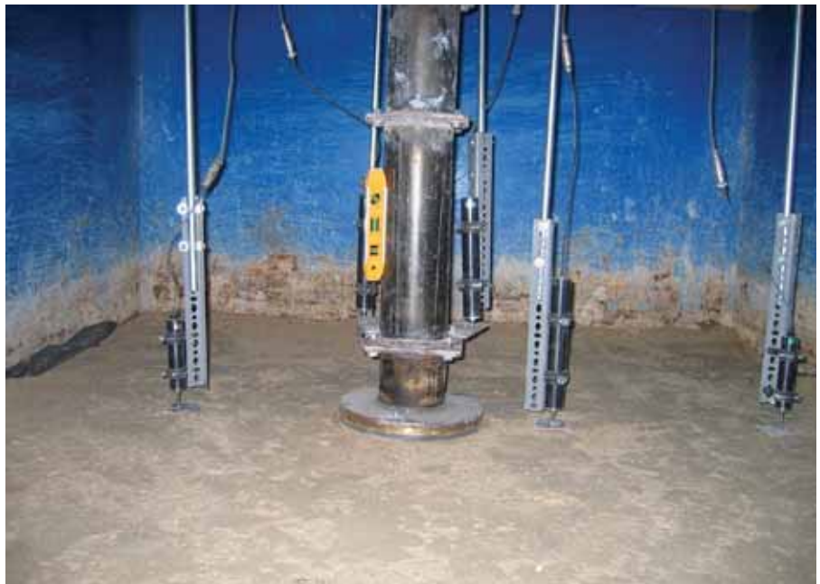
Large-scale plate loading test in the geotechnical test box. The repeated loading tests investigated the effect of infill material on the performance of geocell-reinforced bases.
