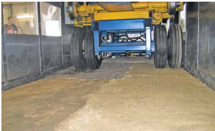
Accelerated pavement testing of unpaved road sections at Kansas State University.
